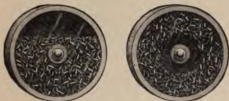
FIG. 105.—The Holtzer-Cabot centrifugal shunt. When at rest the copper granules settle around the end of the spindle. When it is revolved they are thrown out by centrifugal force, thus breaking the shunt circuit.
